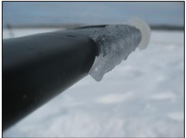
Photo 4. Ice on the horizontal stabilizer leading edge
