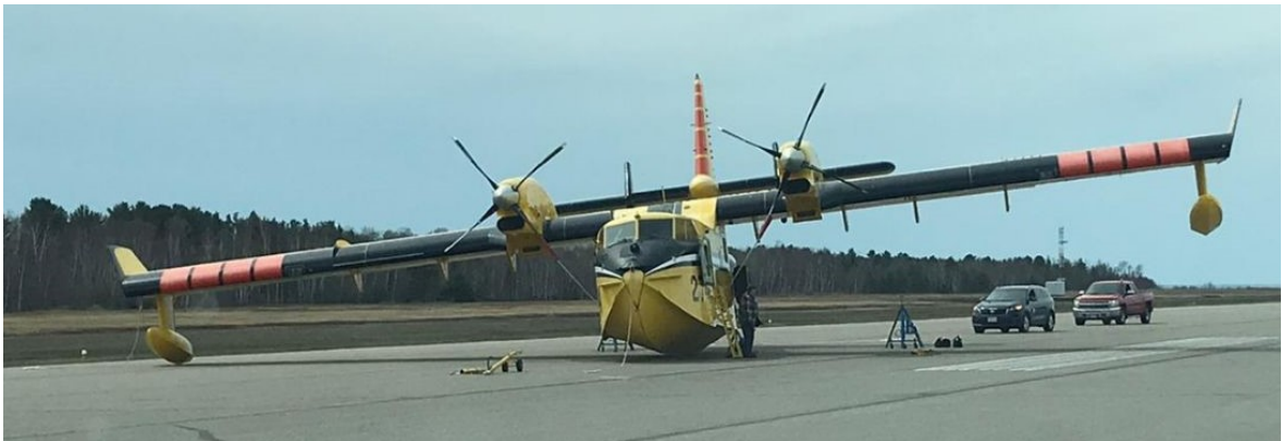
Figure 1. Photo of the occurrence aircraft after the gear-up landing (Source: Province of Ontario, Ministry of Northern Development, Mines, Natural Resources and Forestry)
