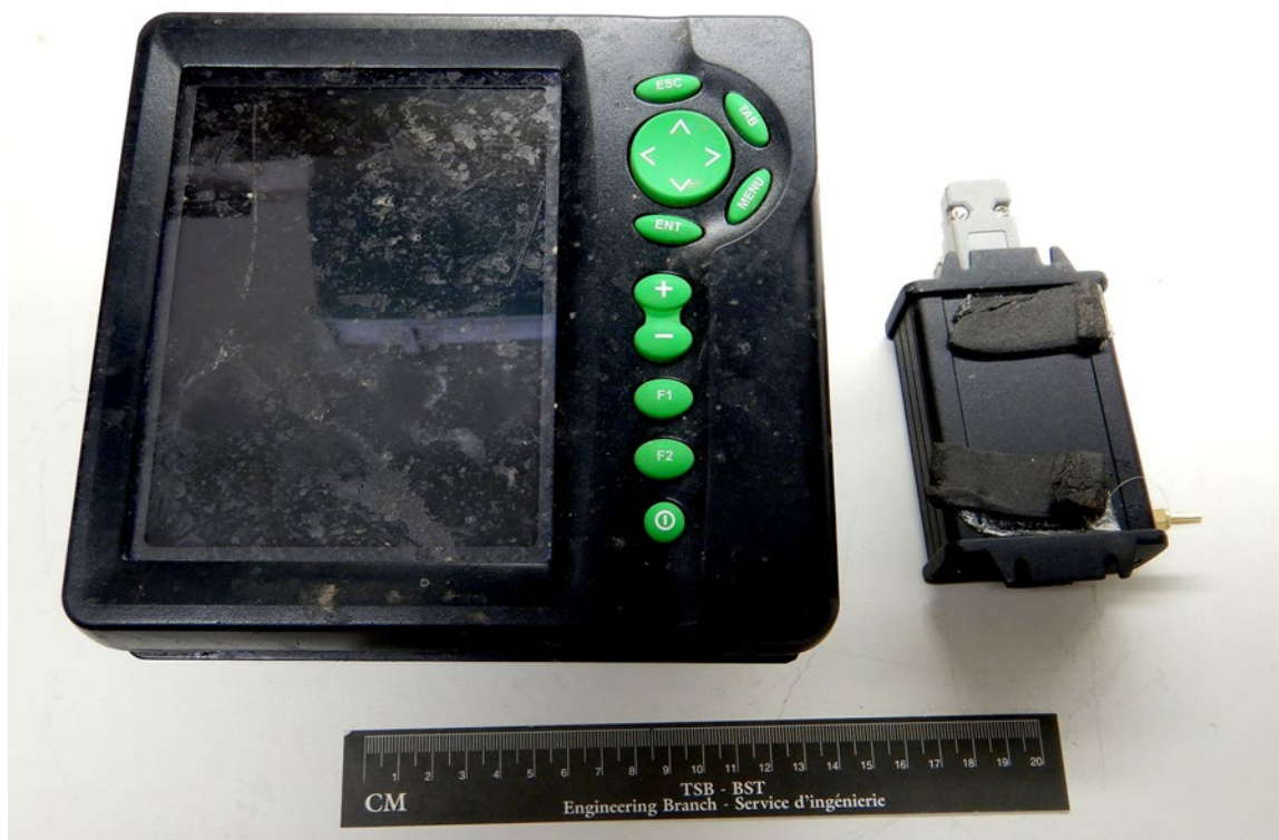
Figure 3. TracMap Flight1 device and GPS antenna recovered from the occurrence helicopter (Source: TSB)
