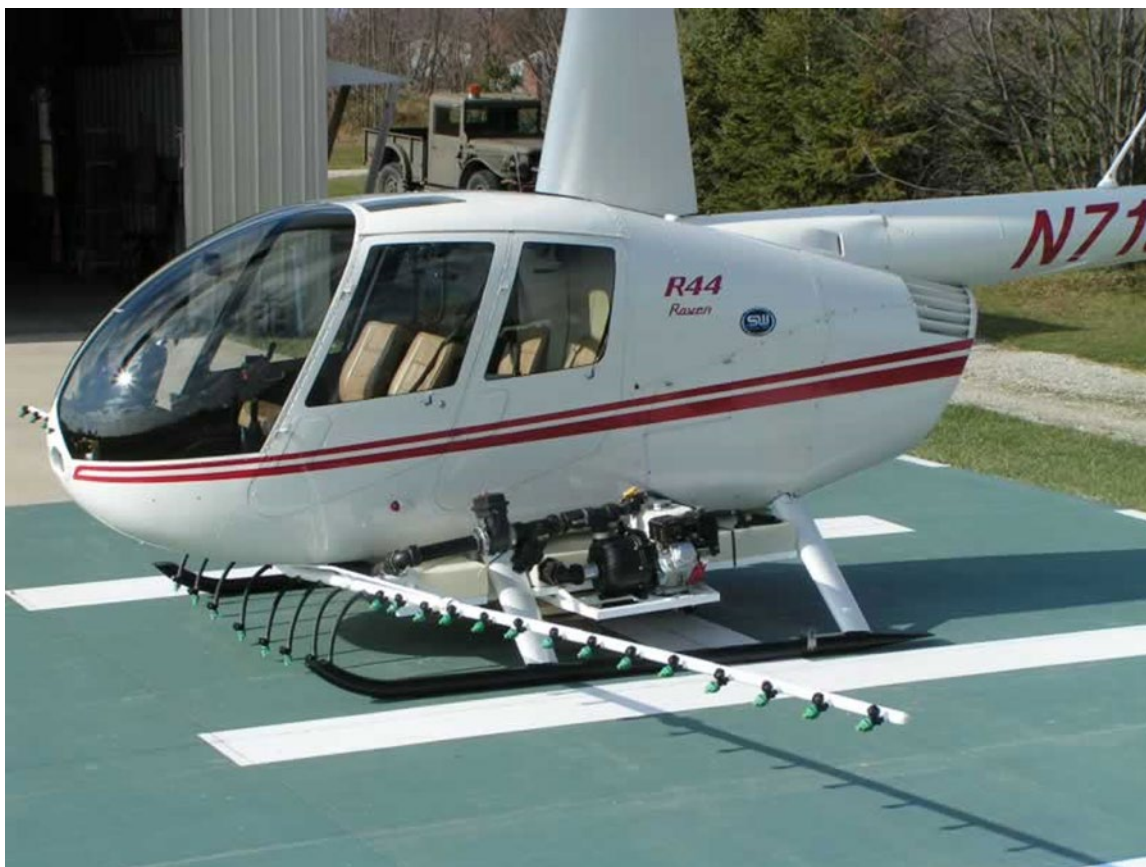
Figure 2. Photo of a Robinson R44 helicopter equipped with the Apollo Spray DTM-4 spray system (Source: Apollo Spray Systems)
