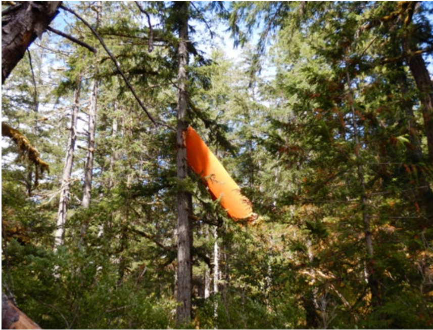
Figure 3. Occurrence aircraft's right wing lodged in a tree (Source: RCMP)
