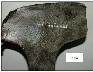
**Photo 2b.** Fracture face A with beach marks in the fatigue crack region
