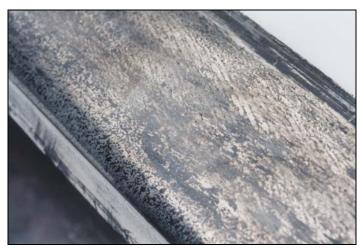
Photo 5. Head checks in larger piece of recovered rail
