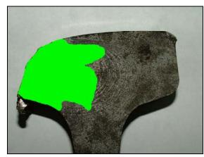
**Photo 7.** The burnished fatigue area (green) of fracture surface A
