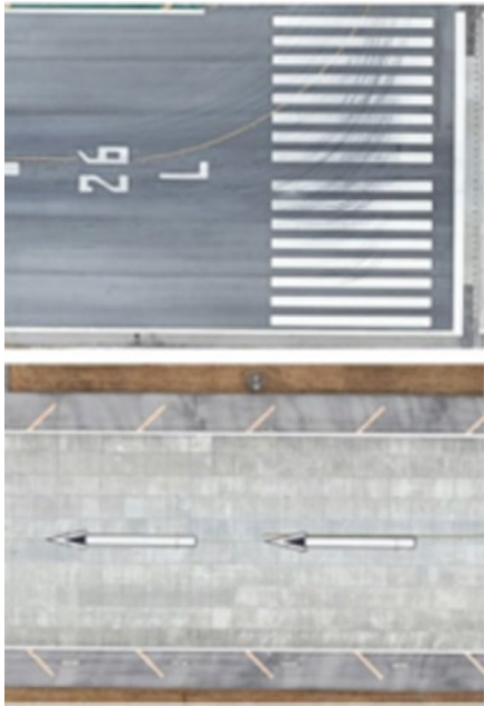
Figure 3. Runway threshold (top) and displaced threshold area (bottom) at Vancouver International Airport (Source: Google Earth)
