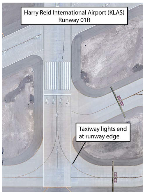
Figure 5. Taxiway lighting at intersection with Runway 01R at Harry Reid International Airport (Source: Google Earth, with TSB annotations)
