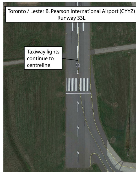
Figure 6. Taxiway lighting at intersection with Runway 33L at Toronto/Lester B. Pearson International Airport (Source: Google Earth, with TSB annotations)
