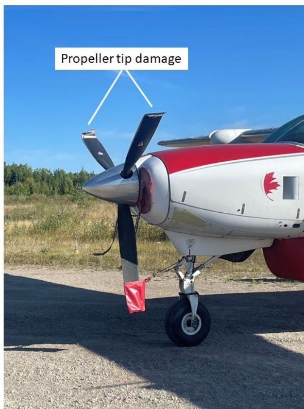
Figure 4. Damage to the propeller blade tips (Source: Superior Airways Limited, with TSB annotations)
