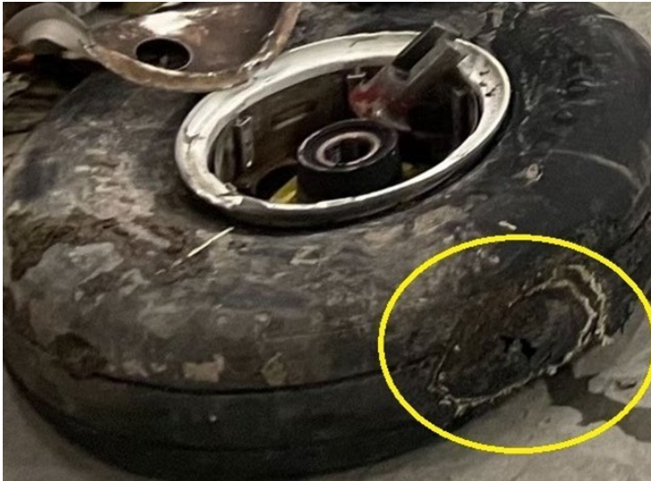
Figure 3. One of the main landing gear tires with damage from the heavy skidding (Source: North Star Air Ltd., with permission)
