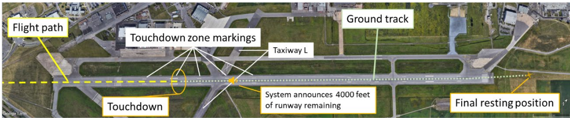
Figure 2. Image showing the touchdown zone markings as well as the aircraft's flight path (dashed line), the touchdown point, the location of the announcement of 4000 feet of runway remaining, the aircraft's ground track (dotted line), and its final resting position (Source: Google Earth, with TSB annotations)
