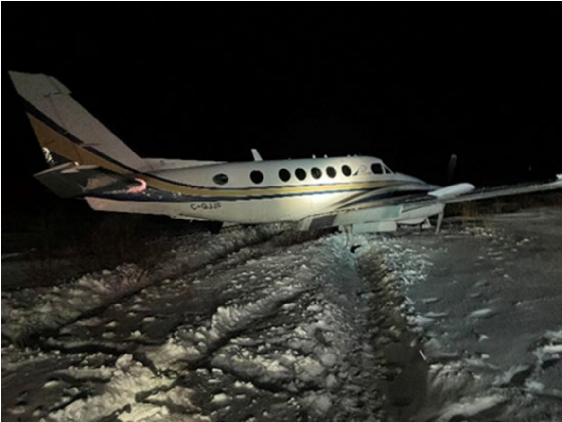
Figure 2. Occurrence aircraft after the lateral runway excursion (Source: Propair)
