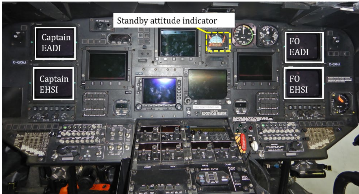
Figure 7. The occurrence helicopter instrument panel highlighting how the smaller size and central location of the standby attitude indicator differ from the larger electronic attitude direction indicator (EADI) and electronic horizontal situation indicator (EHSI) displays that are directly in front of the captain and first officer (FO) (Source: TSB)
