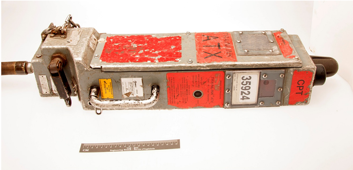
Figure 1: Wabtec Railway Electronics SBU as received
