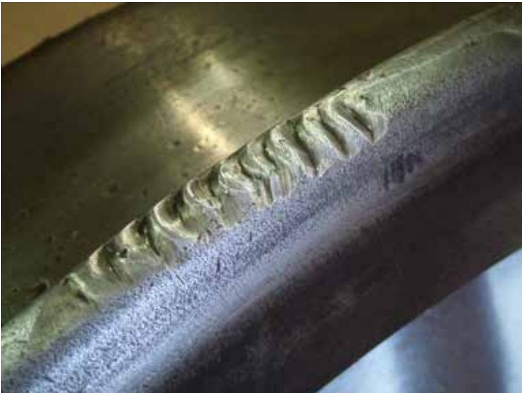
Figure 2: Photograph showing the feature observed on the flange of wheel 83414
