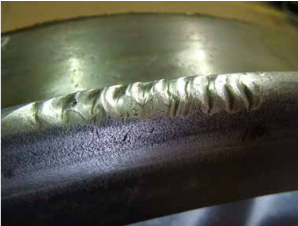
Figure 5: Photograph showing the feature on the wheel flange. Note how the edges have a rounded appearance.
