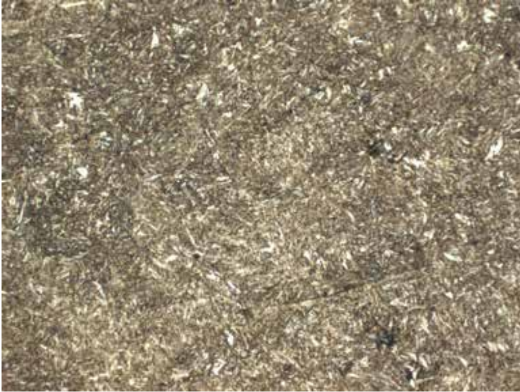
Figure 9: Micrograph showing the fine tempered martensite in the tip area of the wheel flange (Nital etchant, original magnification \times 200 )
