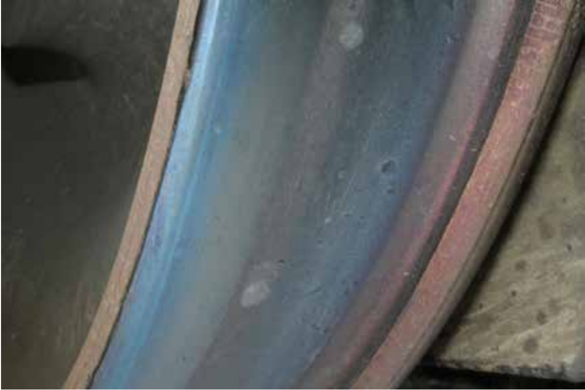
Figure 3: Representative example of wheel tread with \frac{3}{4} blueing
