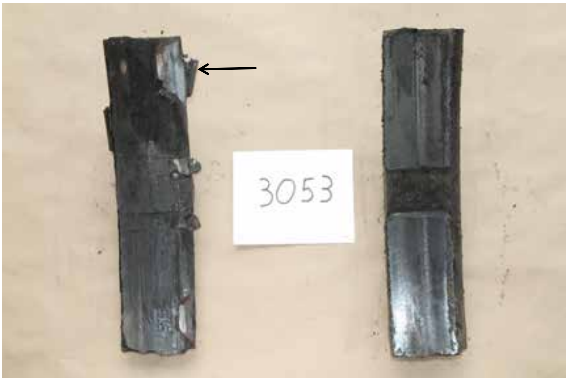
Figure 10: Tread side view of brake shoe lining worn away to backing plate (arrowed)
