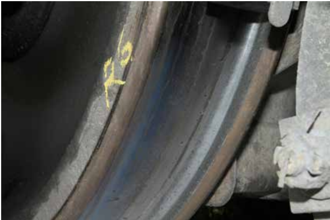
Figure 2: Representative example of wheel tread with \frac{1}{2} blueing
