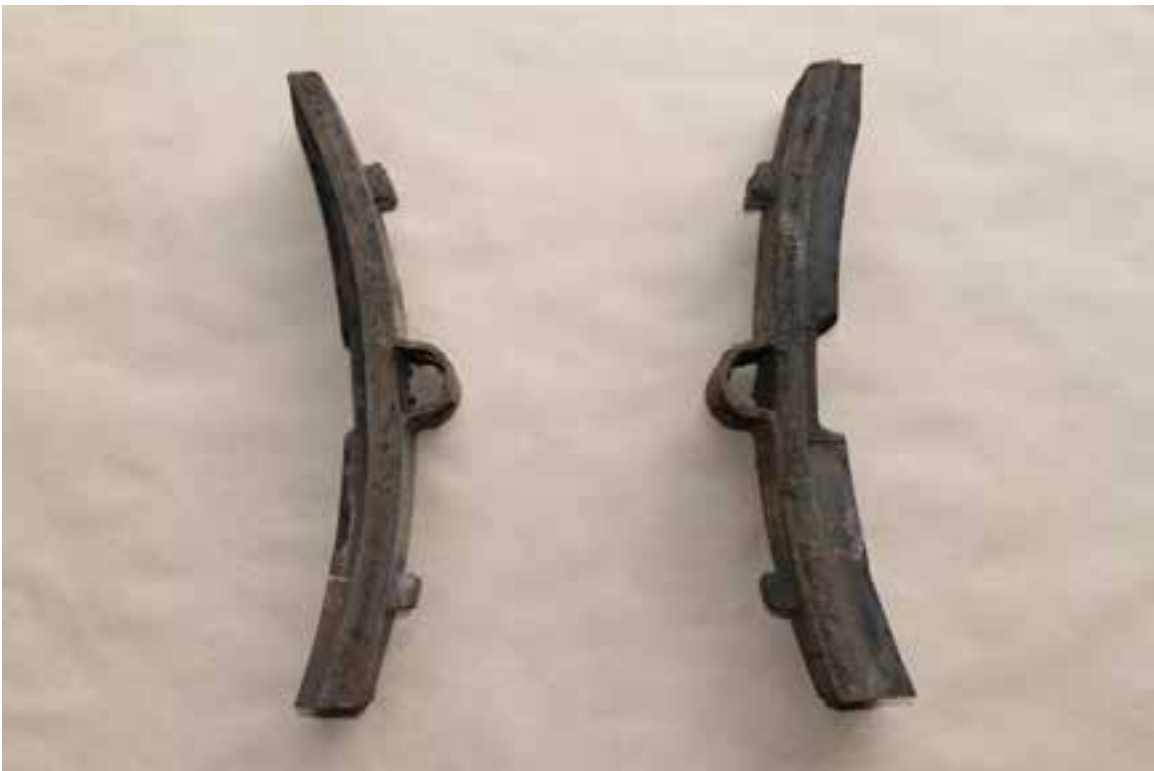
Figure 6: Representative brake shoes showing asymmetric wear
