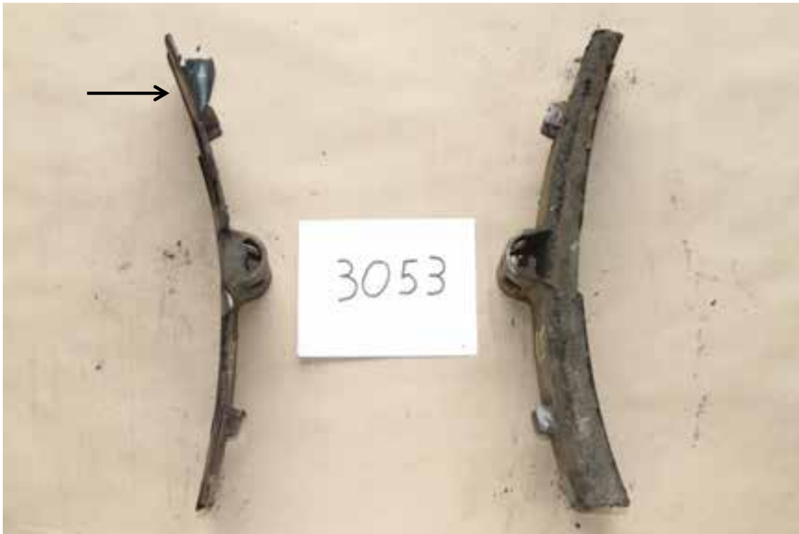
Figure 9: Example of brake shoe with lining worn away to backing plate (arrowed)
