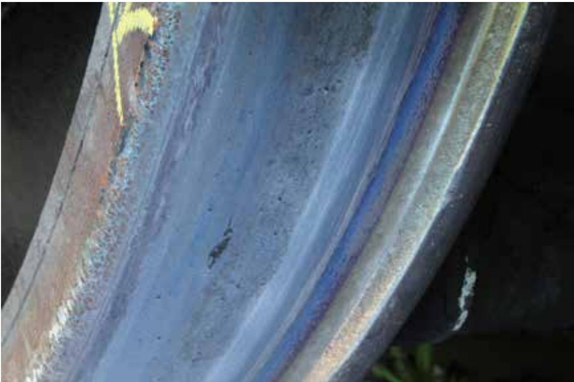
Figure 4: Representative example of full tread blueing including the wheel flange
