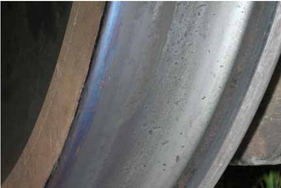
Figure 1: Representative example of wheel tread with \frac{1}{4} blueing
