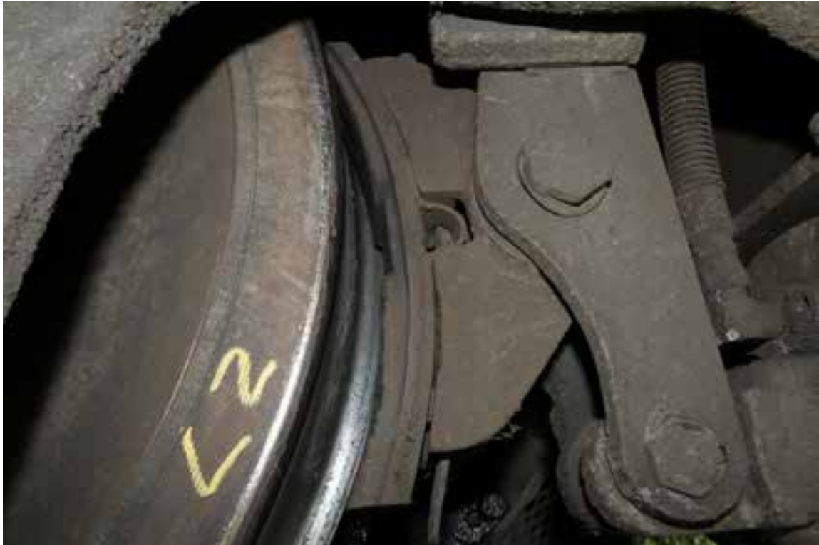
Figure 7: Brake shoe installed showing asymmetric wear
