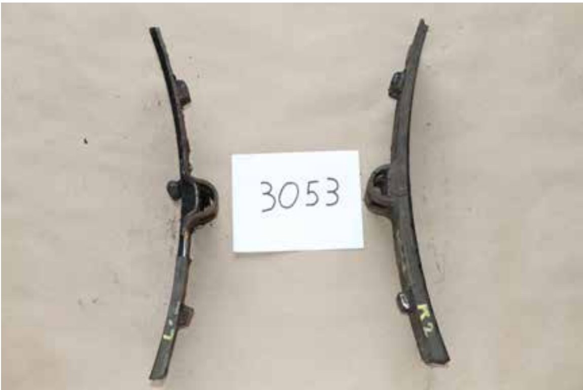
Figure 8: Example of brake shoes with little lining remaining
