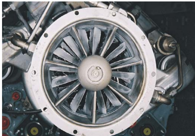
Photo 2. Inlet front support guide vanes and first-stage rotor blades leading edges showing minimal foreign object damage
