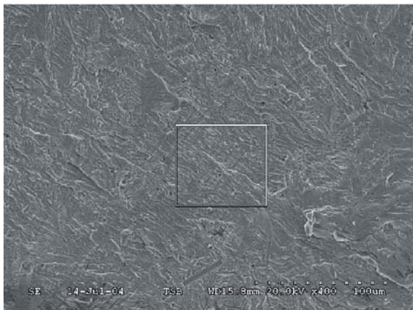
Photo 7. Fracture surface image
