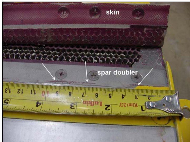
Photo 2. Close-up of blade tip with arrows showing adhesive residue on the spar doubler
