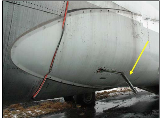
Photo 3. Aft cargo door closed and unlocked
