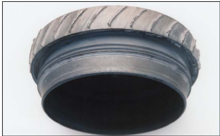
Photo 2. Damaged third-stage compressor wheel
