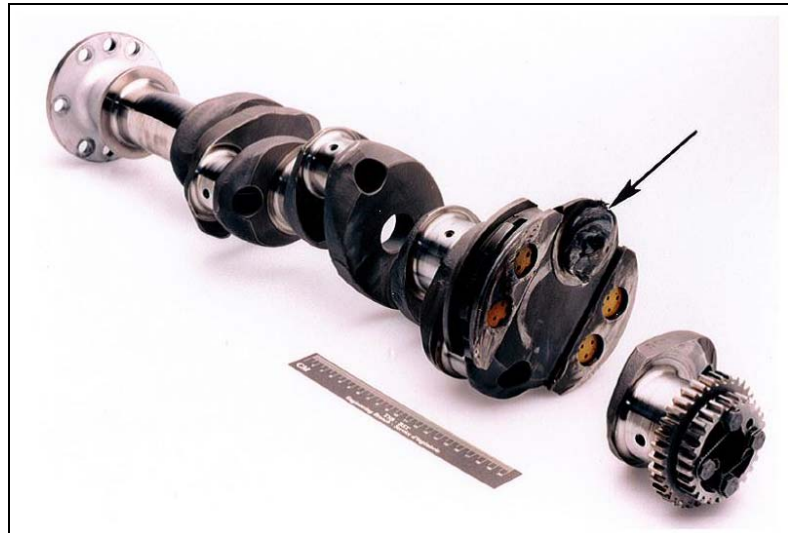
Photo 1. LTSIO-360 crankshaft fracture
