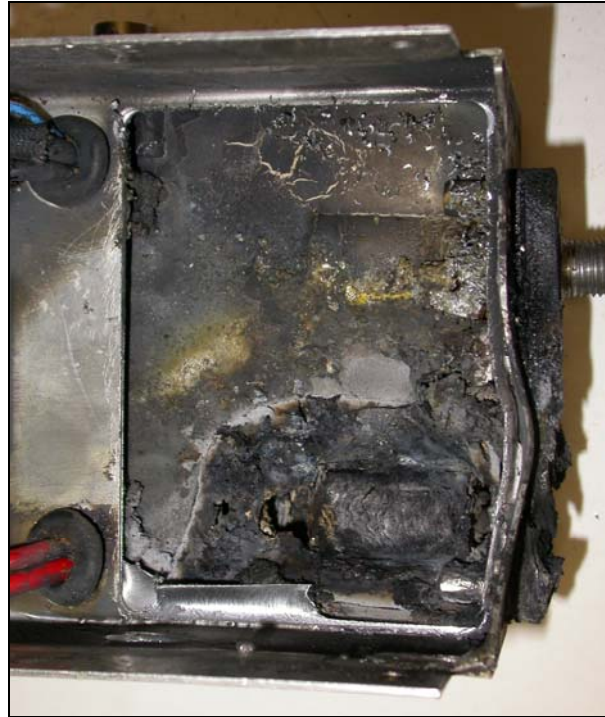
Photo 2. Filter assembly with bottom plate removed
