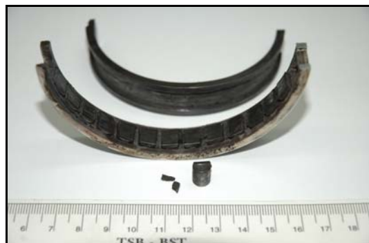
Photo 4. Worn 4.5 Roller Bearing
