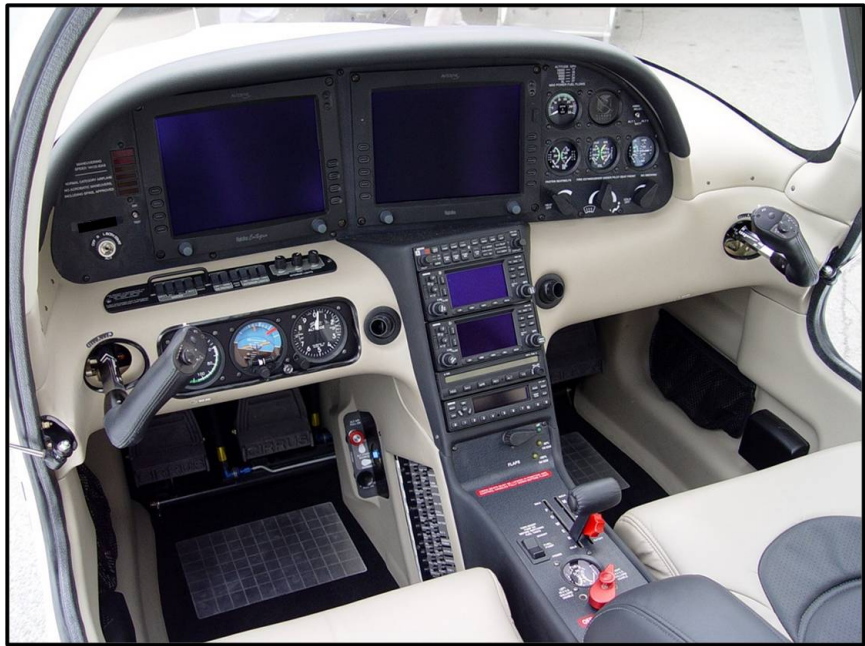
Photo 1. Cockpit and flight controls of an SR22 Source: Steve Pellegrino 2004; Reprinted with permission
