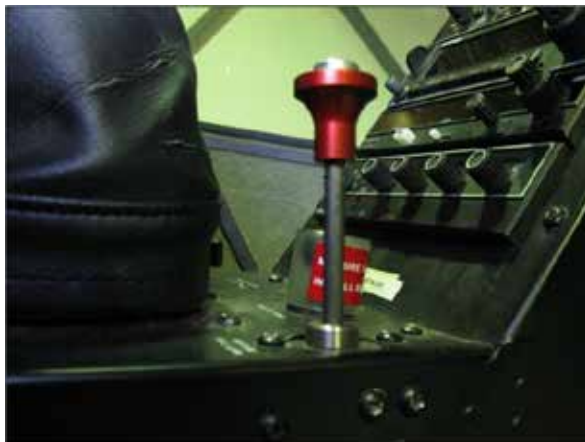
Photo 3. Mixture control in idle cut-off position
