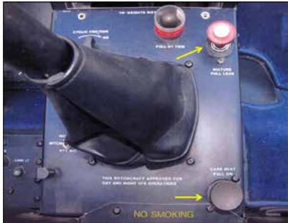
Photo 1. Mixture control top right and carburetor heat control bottom right
