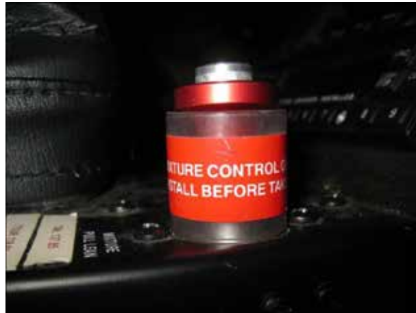
Photo 2. Mixture control with guard installed
