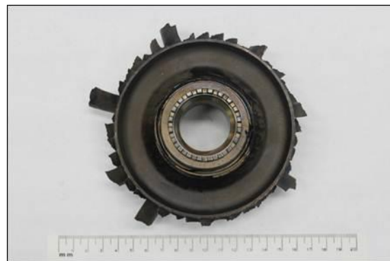
Photo 2. Occurrence third-stage power turbine wheel
