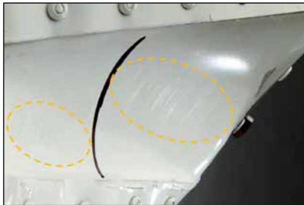
Photo 4. Scratches on aileron rib
