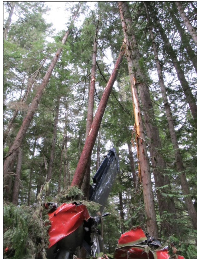
Photo 2. Wreckage and tree strike damage
