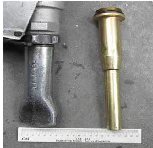
Photo 3. Exemplar flared spout (left) and reduced-diameter (brass) spout
