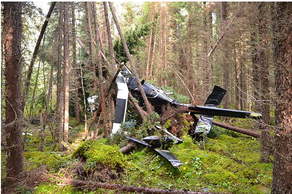
Figure 3. View of C-GHHU from aft left (severed vertical fin visible to the left of tail boom)
