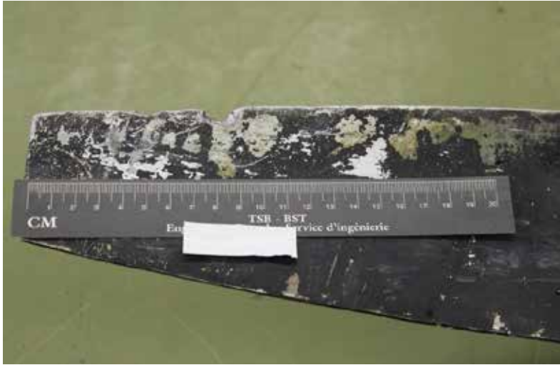
Figure 10. Impact dents on blade 2 of C-FGOI's propeller
