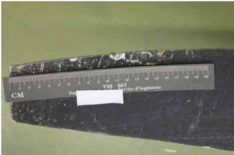
Figure 10. Impact dents on blade 2 of C-FGOI's propeller
