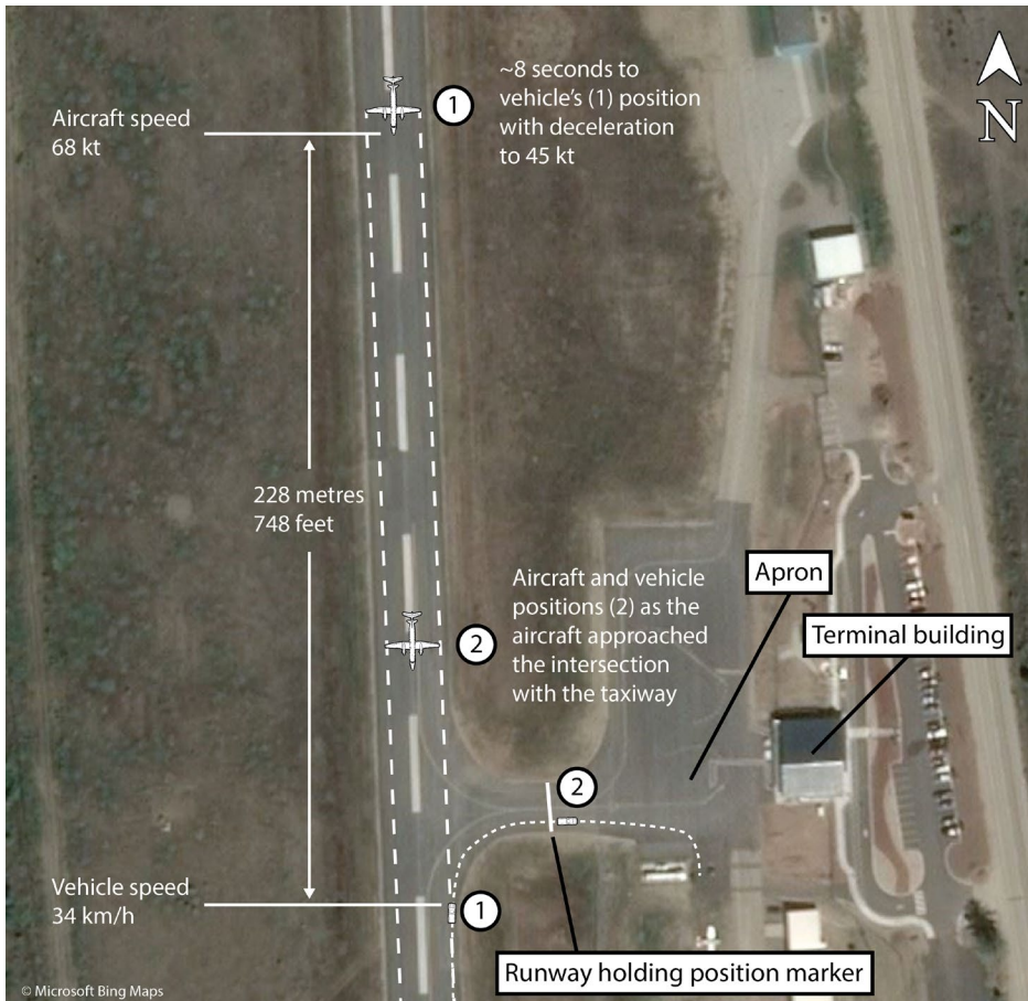
Figure 1. Aircraft and vehicle positions when the aircraft was applying full reverse (1) and as it approached the intersection with the taxiway (2) (Source: Microsoft Bing Maps, with TSB annotations)
