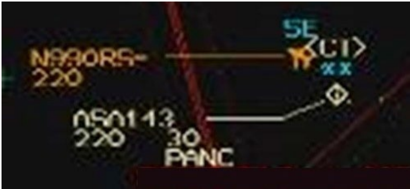
Figure 3. Close-up view of the Canadian Automated Air Traffic System Situation Display showing the Piaggio as 2 targets (Source: NAV CANADA)
