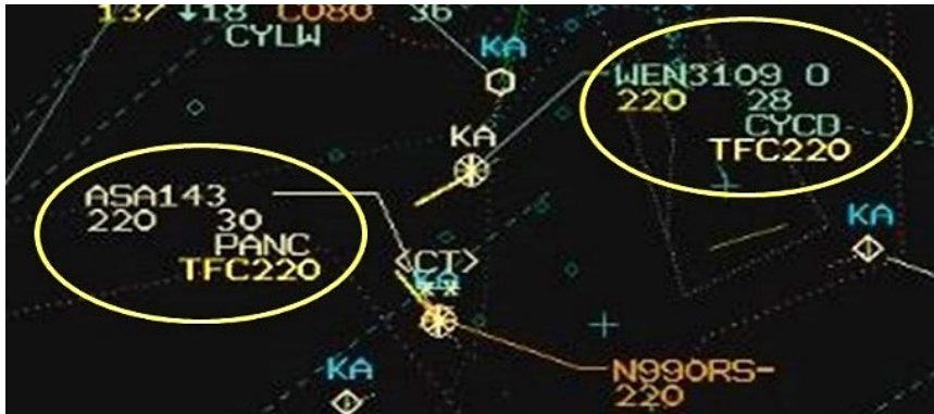
Figure 9. Close-up view of the Canadian Automated Air Traffic System Situation Display with the TFC220 alert for the Piaggio (shown as ASA143) and the Q400 (WEN3109) (Source: NAV CANADA, with TSB annotations)
