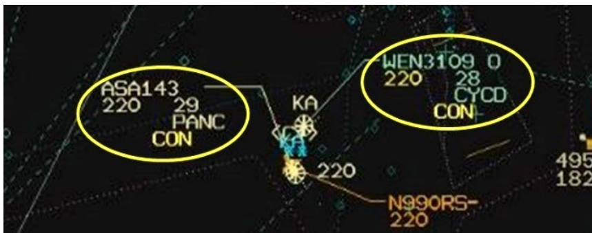
Figure 10. Close-up view of the Canadian Automated Air Traffic System Situation Display showing the 2 occurrence aircrafts' data tags after the TFC220 alert changed to the CON alert (Source: NAV CANADA, with TSB annotations)
