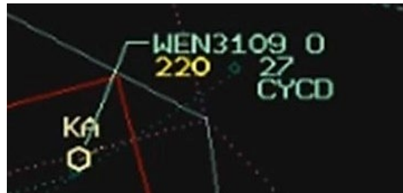
Figure 7. Close-up view of the Canadian Automated Air Traffic System Situation Display displaying the Q400's (WEN3109) correlated target (Source: NAV CANADA, with TSB annotations)
