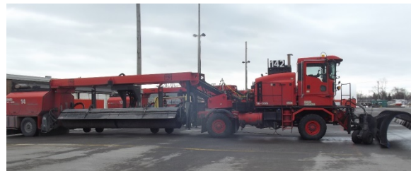
Figure 1. Snowplow-sweeper CHA142, an HT tractor with plow and XT tow-behind broom (Source: TSB)
