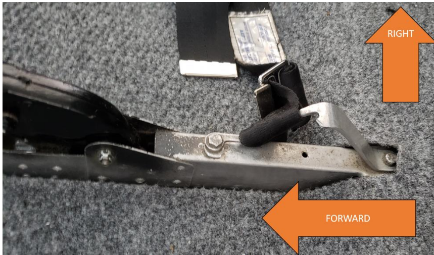
Figure 3. Lap belt centre bracket on the occurrence aircraft (Source: TSB)
