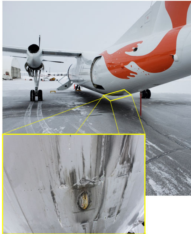
Figure 2. Rear view of another DH8C and view of the damage to C-GXAI (Source: TSB)
