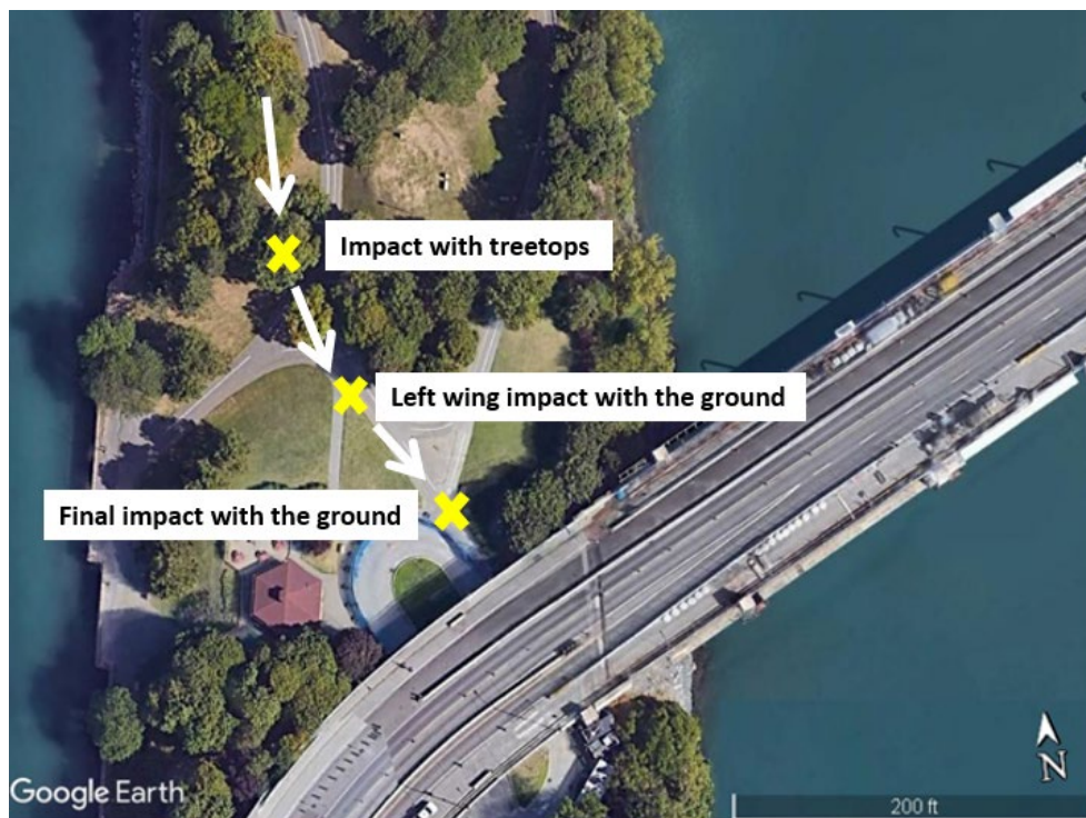
Figure 2. Image showing the occurrence aircraft's impact sequence (Source: Google Earth, with TSB annotations)
