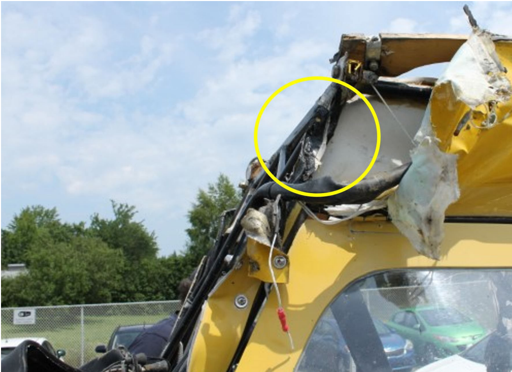
Figure 3. Photo of the damage to the left windshield post caused by the collision with the cable (Source: TSB)
