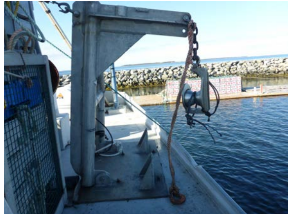
Photo 3. Overhead block in raised position
