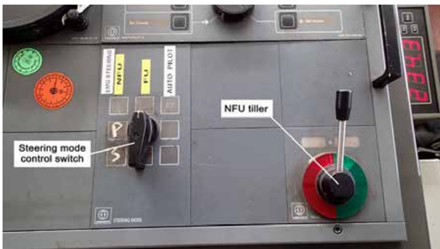
Figure 6. Non-follow-up tiller of the MSC Monica
