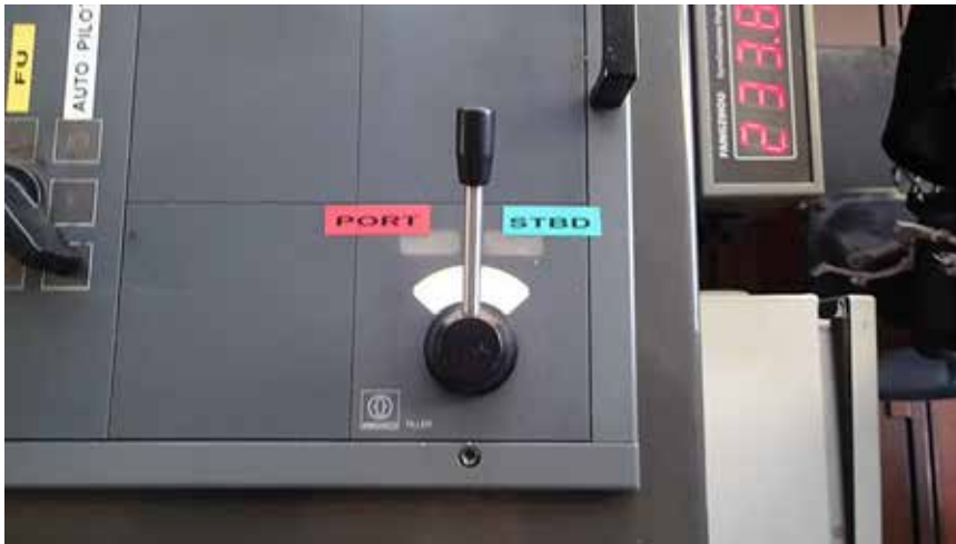
Figure 9. Non-follow-up tiller of the MSC Monica without the plastic disk, but with the new colour-coded labels
