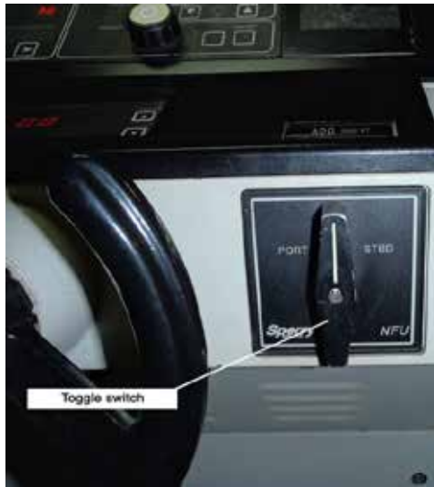
Figure 4. Non-follow-up tiller – Toggle switch
