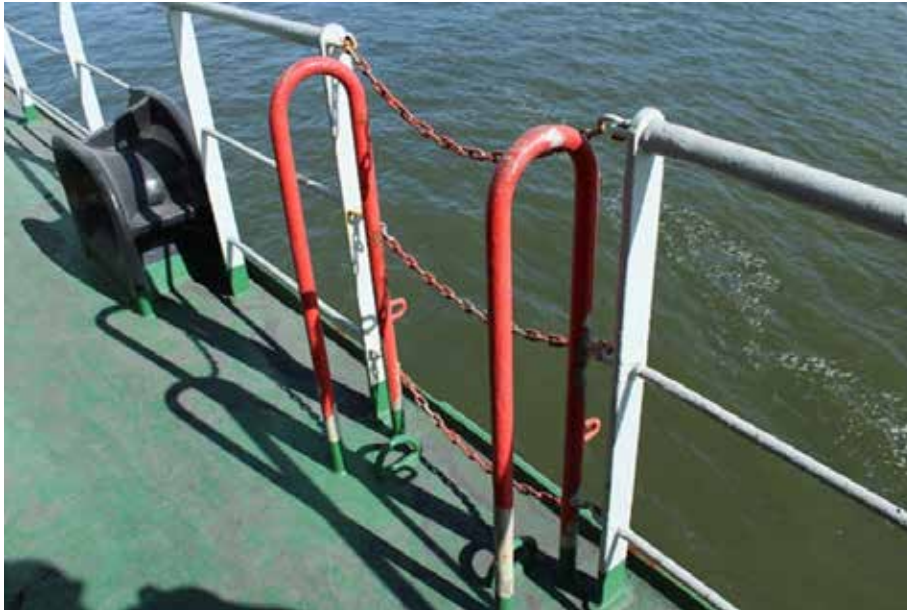
Figure 4. Pilot gateway on board the Amazoneborg
