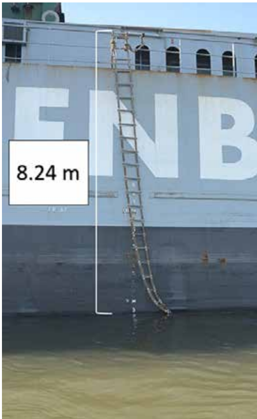
Figure 3. Side view of the Jacob's ladder, indicating height at the time of the occurrence (8.24 m) (Source: Louise Charbonneau/Sûreté du Québec, with TSB annotations)
