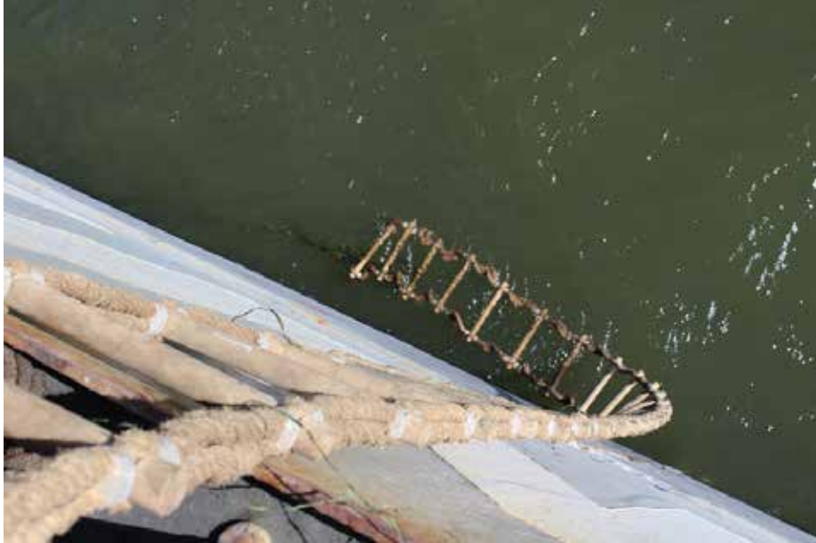
Figure 2. Top view of the Jacob's ladder hanging over the port side of the Amazoneborg, near the amidships draft marks
