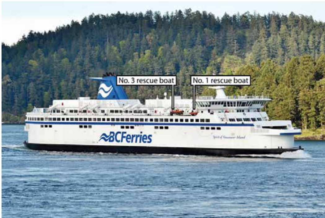
Figure 1. The Spirit of Vancouver Island and its starboard-side rescue boats (Source: British Columbia Ferry Services Inc., with TSB annotations)
