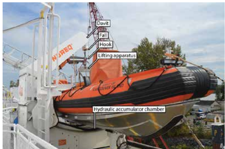
Figure 2. A rescue boat similar to the occurrence rescue boat, with the same type of davit
