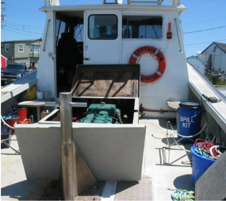
Figure 2. View of the wheelhouse from aft showing raised coaming around engine compartment and one of the hatch covers (Source: Third party, with permission)
