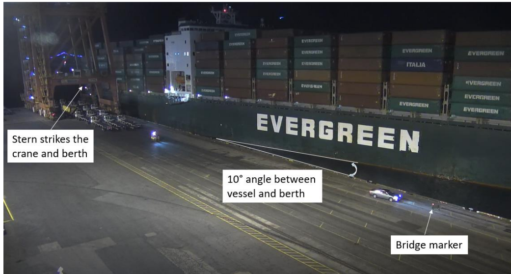
Figure 5. Capture from the closed-circuit television footage of the Ever Summit at the time of the striking (Source: GCT Canada, with TSB annotations)
