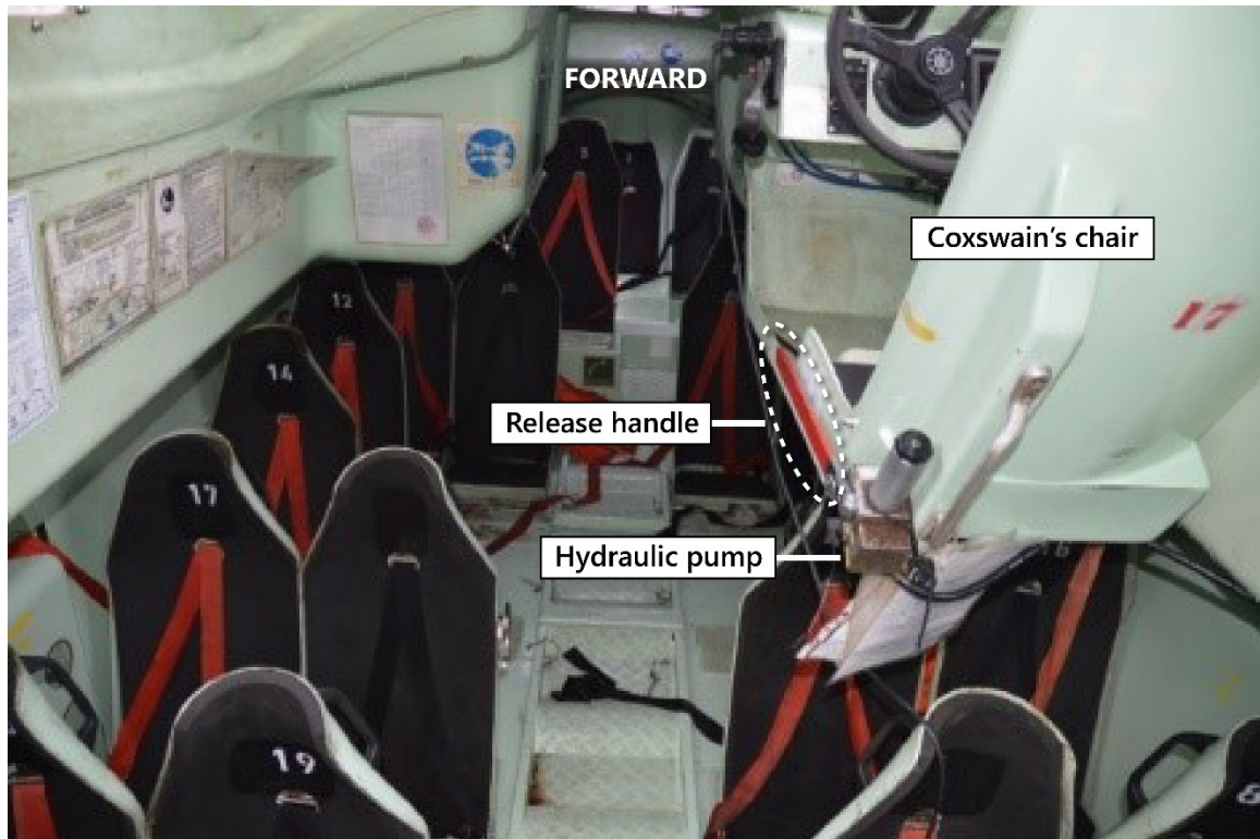
Figure 5. View inside lifeboat showing release handle beside coxswain's chair (Source: TSB)
