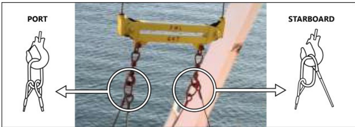
Figure 4. Photo and diagram showing how the slings were attached to the hooks during the occurrence drill (Source: Apollonia Lines S.A., with TSB annotations)
