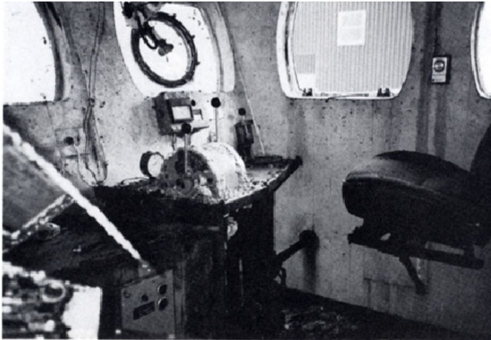
Bridge control in forward starboard corner of wheel-house.
