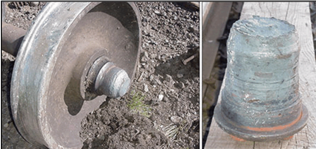
Photo 2. Photos of L3 wheel and burnt-off journal stub from car XPWX 2007 showing damage resulting from an overheated roller bearing.
