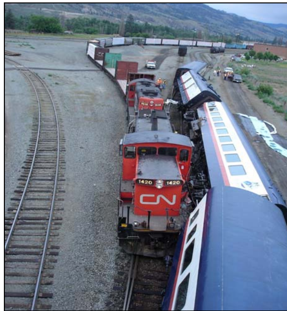
Photo 1. Derailed passenger cars
