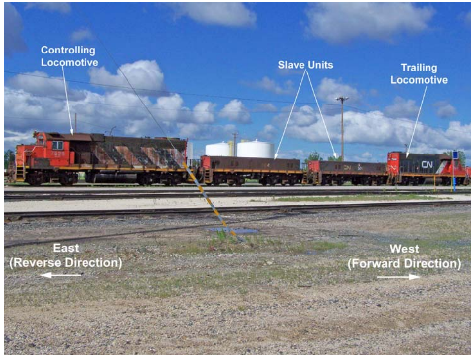
Photo 2. Normal hump set configuration at Symington Yard
