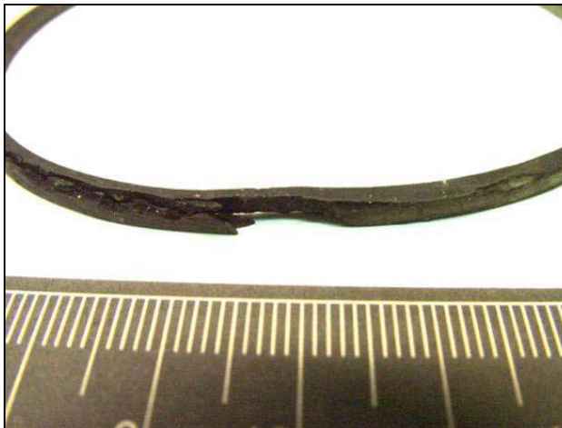
Photo 3. Damaged O-ring gasket
