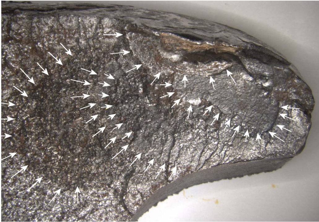
Photo 2. Arrows show crack arrest lines. Progressively less corrosion and a rougher surface topography was visible further away from the gauge corner.
