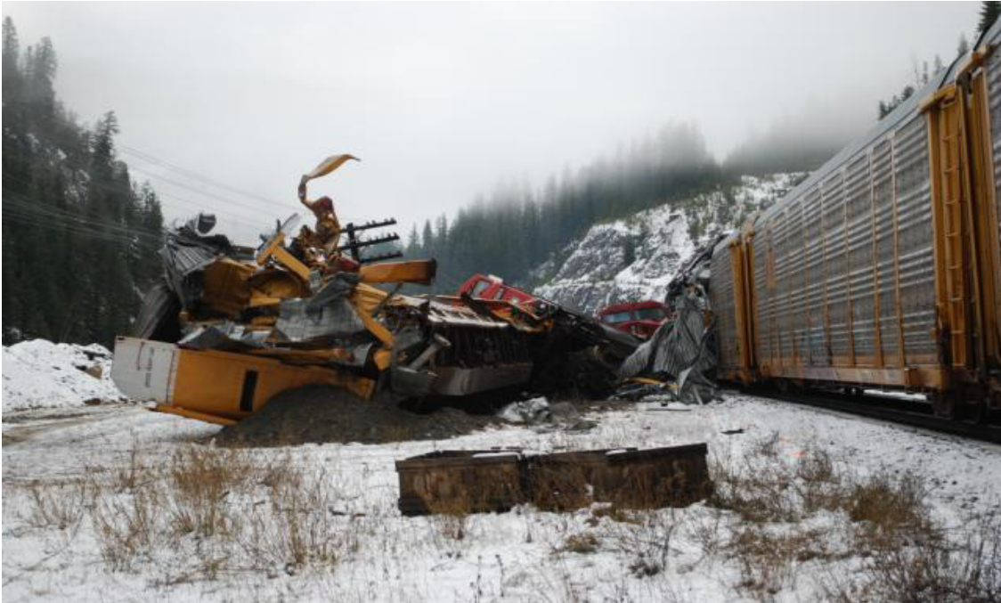
Photo 1. Derailment damage of auto cars from Train 110 and locomotives from Train 355
